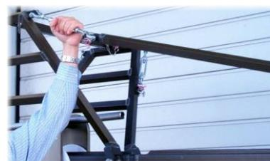
Tensioning the turnbuckle
