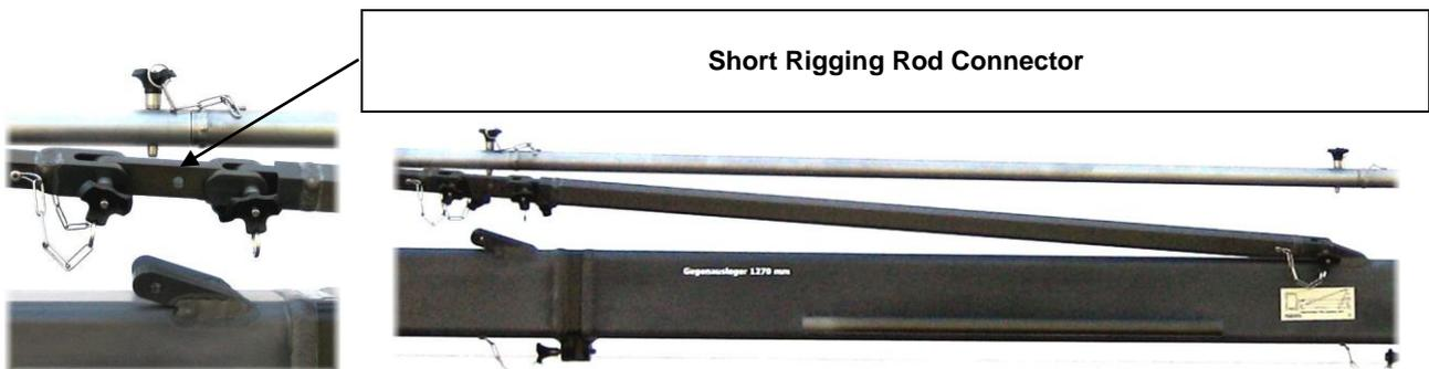
6. After the complete rigging system has been assembled, hand tighten the turnbuckles until the rigging rods are taut. The turnbuckles can be secured with locking nuts. Make sure that the rigging is absolutely straight. For this case the Adjustable Rigging Rod Support has to be adjusted in a proper way.
