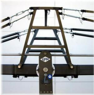
Large Rigging Harness for double Rigging
