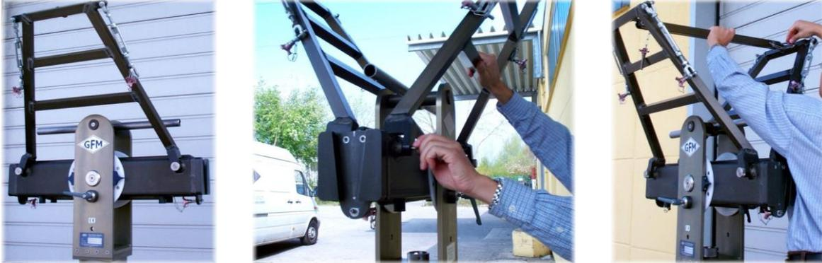
Mounting the Standard Rigging Harness
