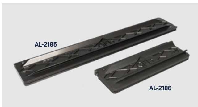
AL-2185 GF-Camera Support Plate 60 Dimensions: 60 x 9.7 x 2.7 cm / 23.6" x 3.8" x 1" Weight: 1.7 kg / 3.7 lbs AL-2186 GF-Camera Support Plate 30 Dimensions: 30 x 9.7 x 2.7 cm / 11.8" x 3.8" x 1" Weight: 0.86 kg / 1.9 lbs
