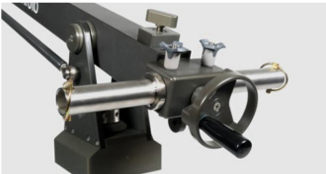
Its counterweight arm can be steplessly adjusted by a crank and extended up to a max. of 100 cm. A user-friendly brake attached to the end of the GF-Mini Jib also serves as friction, depending on the tight-ening torque. Most Jib Arm components are made of aluminium and have a very hard and durable surface protection (Hart-Coat®).
